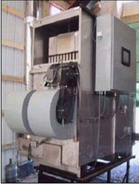
Figure A.4.4: Rear view of completed prototype showing commercial-design controls system on left side of unit
