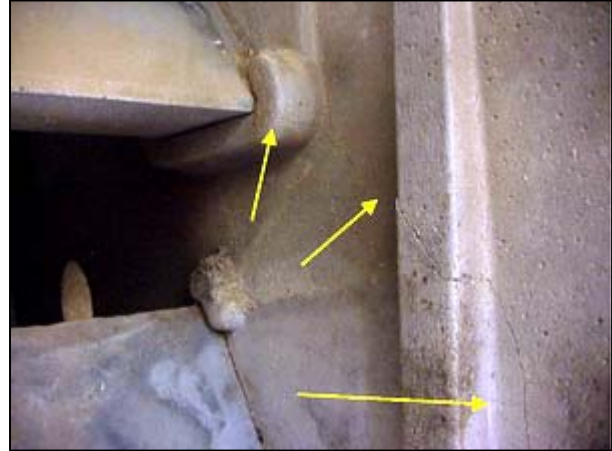
Figure A.3.8: Cracks in ceramic components
