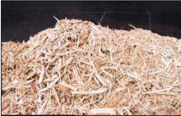
Figure A.4.7: Shredded woody residue (from a RotoChopper) used by EP/WM for testing purposes
