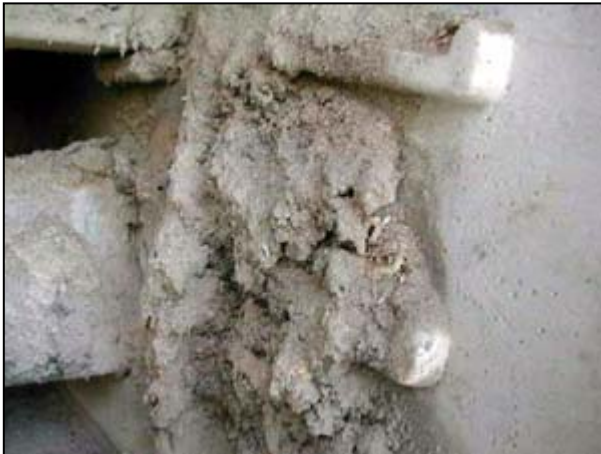
Figure A.3.9: Slagging from litter testing
