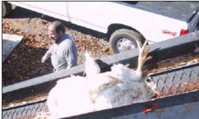
Figure A.4.9: Mortality going up the belt conveyor to the fuel intake chute during mortality incineration test
