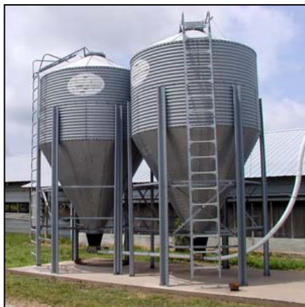
Figure 36: typical pre-fabricated grain silos that can be used for storing pellet fuel
