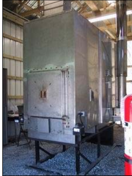
Figure A.4.5: Front view of completed prototype with metal skin installed and exhaust stack on right side of unit
