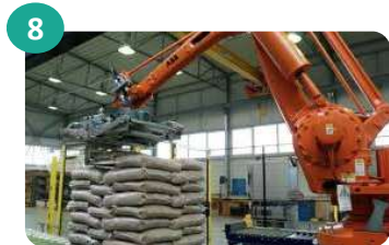
8 Bags are automatically palletized (robot or dedicated palletizer)
