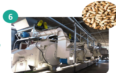
6 Sized and dried material is processed through a pelletizer using rotating rolls and dies to form the pellet
