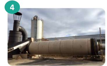
4 Material is dried from "green" state (~40% moisture) to desired moisture content (~10 - 15%)
