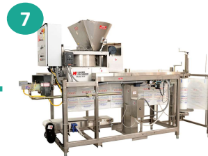
7 Pellets are bagged by an automated form, fill and seal machine in either 10, 20 or 40 pound bags
