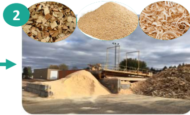
2 Residuals can be in the form of chips, sawdust or shavings and are stored until material is processed
